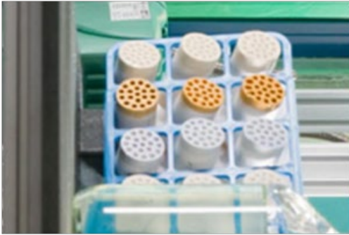
Fig: Ceramic UF membranes for diesel/water separation.
